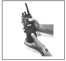
Figure 9 - Removing the Battery Pack
